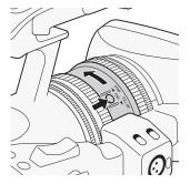
2 Press the PUSH button (unlock focus mode ring button) on the focus mode ring and turn the ring toward AF/MF.
